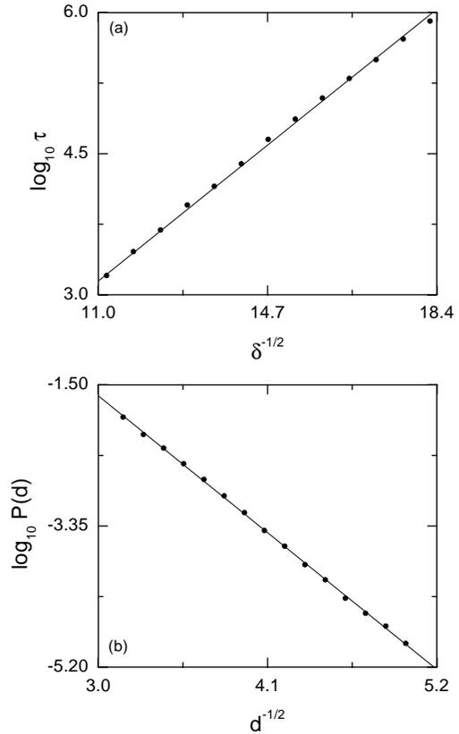
Fig. 3. (a) Plot of  $\log_{10} \tau$  (where  $\tau$  is the average lifetime of a chaotic transient) versus  $\delta^{-1/2}$  (where  $\delta$  is the mismatching parameter) for  $a = 1.71$  and  $b = 1.02$ . (b) Plot of  $\log_{10} P(d)$  (where  $P(d)$  is the divergence probability) versus  $d^{-1/2}$  (where  $d$  is the distance from the  $y = 0$  line) for  $a = 1.71$  and  $b = 1.02$ .
