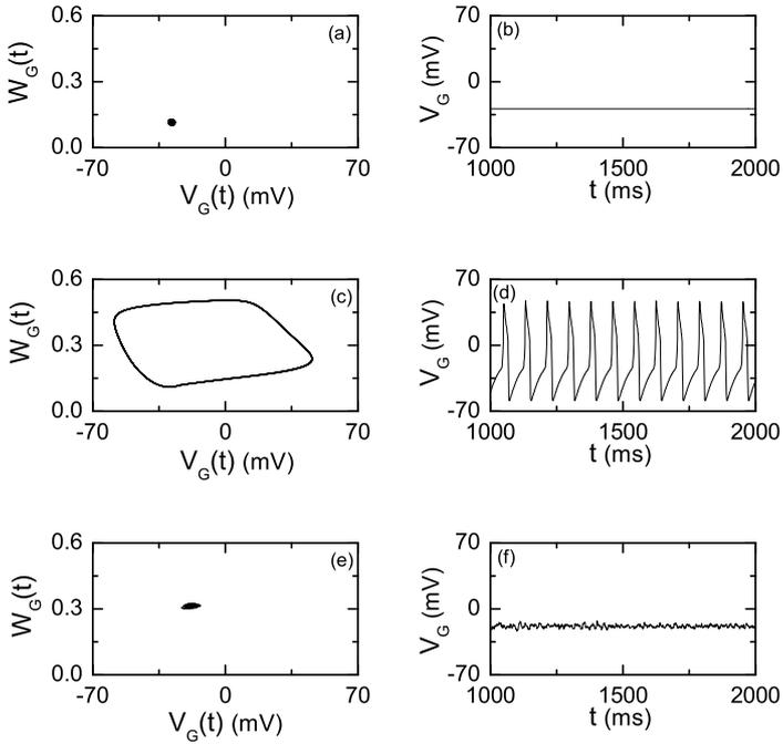
Fig. 1. Incoherence-coherence-incoherence transition for  $N = 10^3$  and  $J = 50 \mu\text{A}/\text{cm}^2$ . Phase portraits of the global state [i.e., lots of  $W_G(t)$  versus  $V_G(t)$ ] and the time series of the global potential  $V_G(t)$  for (a) and (b)  $D = 0.1 \mu\text{A} \cdot \text{ms}^{1/2}/\text{cm}^2$ , (c) and (d)  $D = 0.3 \mu\text{A} \cdot \text{ms}^{1/2}/\text{cm}^2$ , and (e) and (f)  $D = 30 \mu\text{A} \cdot \text{ms}^{1/2}/\text{cm}^2$ .
